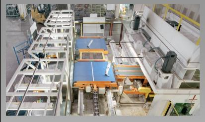
Transfer press cell application. The fast shuttle system gives operators two to three times more time to do an initial online inspection of each part, without compromising cycle rates.
