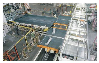
In this typical three station application, a two-position reciprocating shuttle always has an empty side standing ready at the run-out conveyor to pick up the next part while the other side of the shuttle delivers a part to an unload station. Parts can be passed through to a center station without being shuttled.
