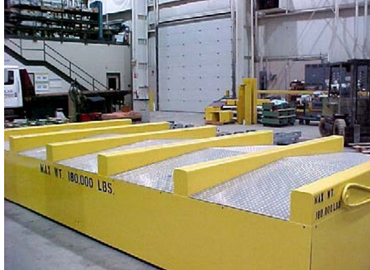
TOP LEFT Atlas "Shuttle Buggy" Transfer Carts which operate in pairs (one powered unit and one nonpowered unit) move railcars through the assembly process for a Canadian based manufacturer.
